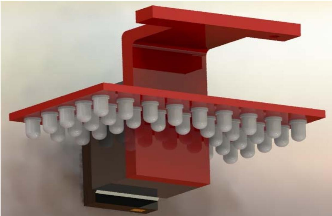
Figure 11: CAD model of LED array on extruder head
