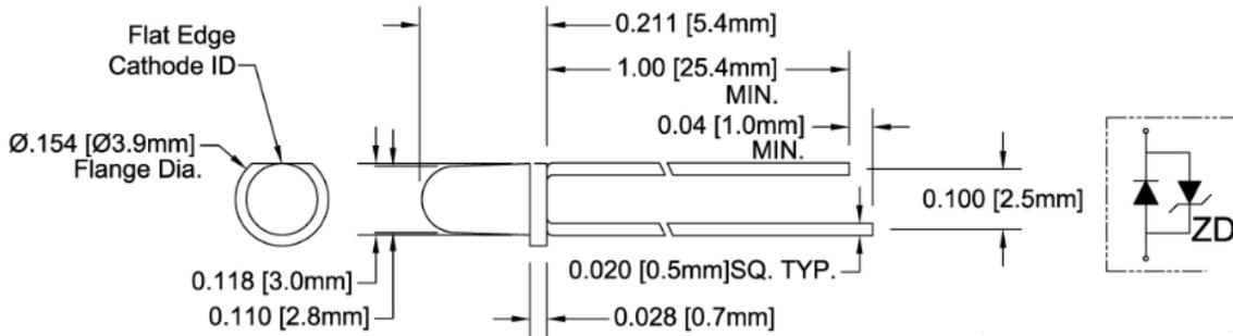
Figure 8: Drawing of LED
