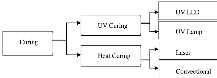
Figure 5: Various methods of curing
