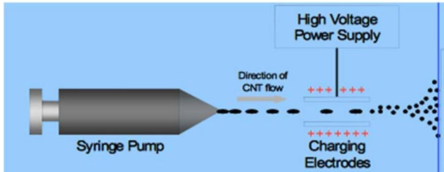
Figure 2: CNT alignment with electrodes
