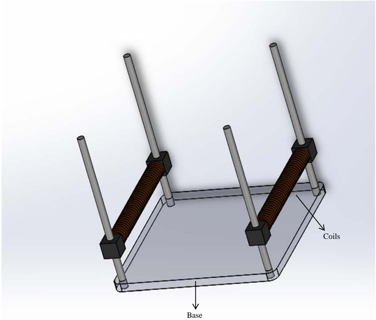
*Figure 10: CAD model of potential alignment field setup*
