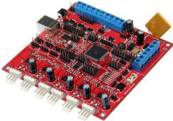
Figure 4: RepRap Arduino Mother Board
